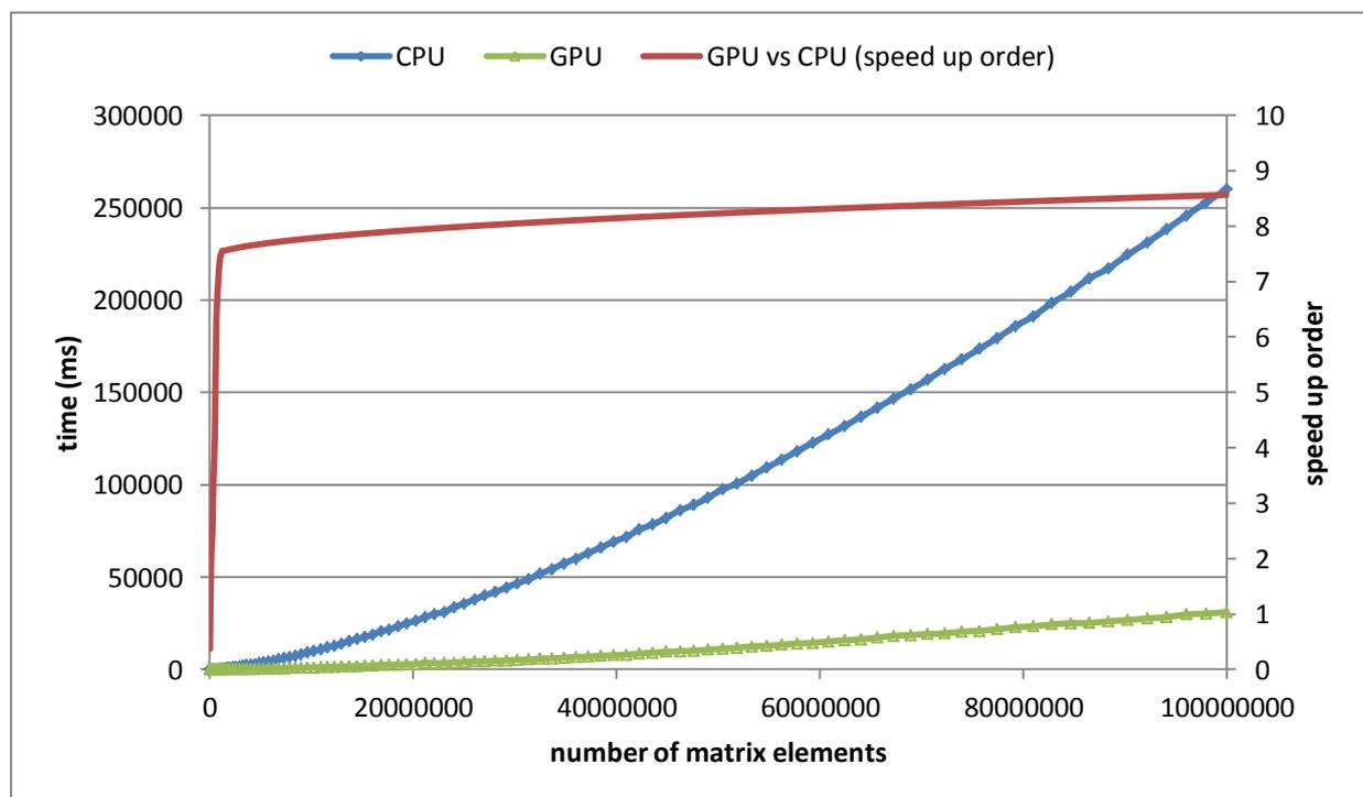
Figure 1. Acceleration of solving the inverse problem for ECT in relationship to the number of the coefficient matrix elements.
