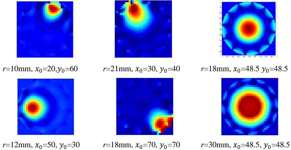
**Fig. 5** Examples of different positions and different radii of phantoms considered in the simulation
