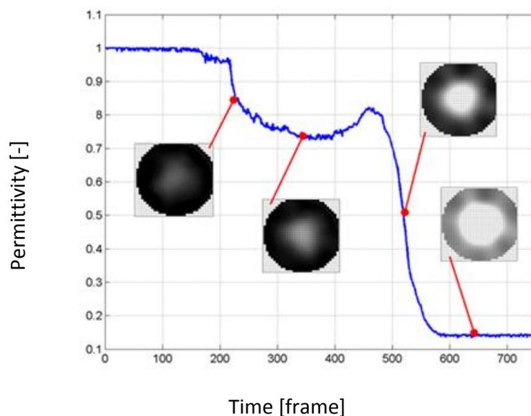
**Fig. 2** Changes of the material concentration (permittivity) distribution inside a sensor (Grudzien et al., 2006)
