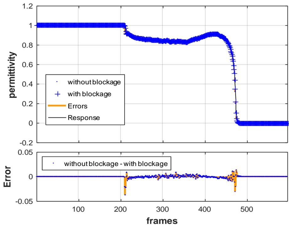
**Fig. 9** Predicted changes of the funnel concentration and obtained errors for the sensor's height of 45mm in the case of the blockage.
