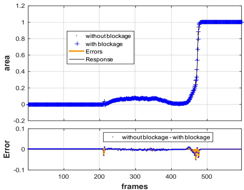
**Fig. 10** Predicted changes of the funnel area and obtained errors for the sensor's height of 45mm in the case of the blockage
