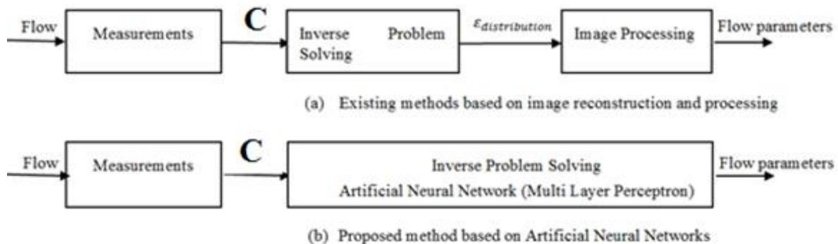
**Fig.** Błąd! W dokumencie nie ma tekstu o podanym stylu. *Different approaches to determine the flow parameters from capacitances data: (a) An existing methods based on image processing and reconstruction, (b) The proposed method based on Artificial Neural Networks*
