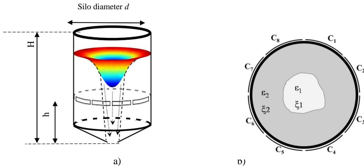
**Fig. 1** Geometrical model of the silo, a) a simplified diagram of emptying the silo - funnel flow, (Grudzien et al., 2006), b) Geometrical modelling of hopper flow in cross section. The set of estimated parameters  $\eta = \{\xi_1, \varepsilon_1, \xi_2, \varepsilon_2\}$ , (Romanowski, Grudzien and Williams, 2006); where:  $H$  – the silo height,  $h$  – the height of ECT sensor position over the silo outlet.
