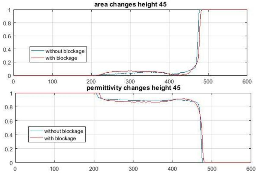
**Fig. 8** Changes in area and permittivity for two cases of the funnel flow: with and without the blockage with the same height of the sensor ( $h=45\text{mm}$ ).
