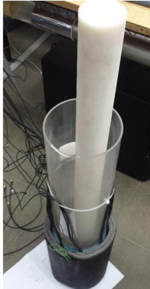
**Fig. 6** A physical model of a cylindrical flow process – a pipe with the object inside and ECT sensor with 8 electrodes placed around
