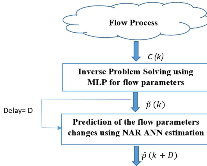
**Fig. 7** Proposed ANN-based approach for flow parameters estimation and prediction
