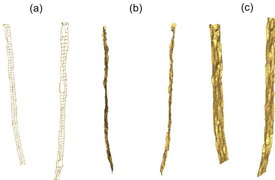
*Figure 3. Three-dimensional edge reconstruction of funnel flow boundary: (a) creating 3D grid (b) front view after hole closed (c) side view after hole closed.*
