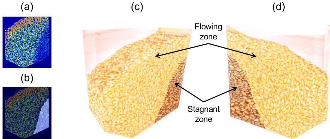
*Figure 5. Volumetric segmentation with the modified u-net model. (a) The absolute difference between two successive original scans of rice grains flow (b) predicted segmentation. The network predicted dense segmentation (c) left side (d) front side view.*
