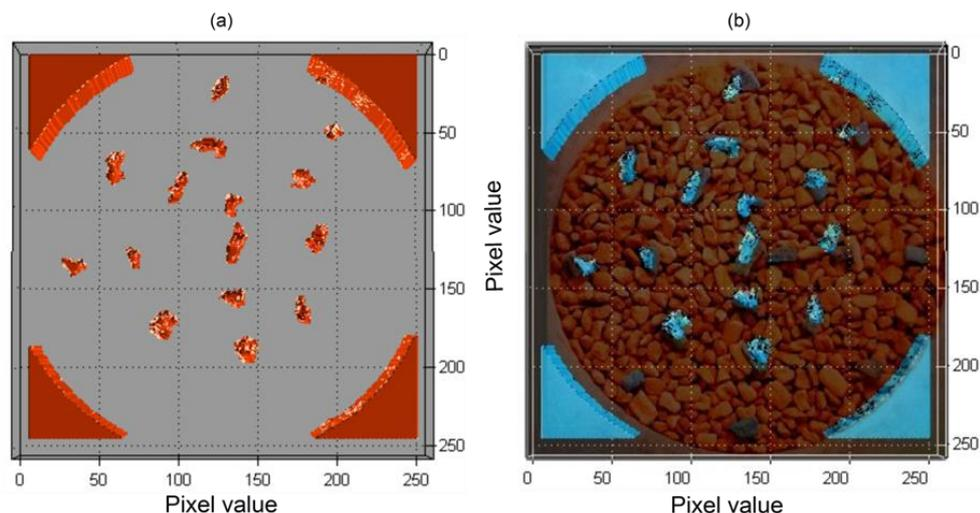
*Figure 1. 3D view of segmented tracer particles at scanning height of 800 mm. (b) Top view photo was taken before discharging during the experiment at silo height of 900 mm superimposed with figure-a.*
