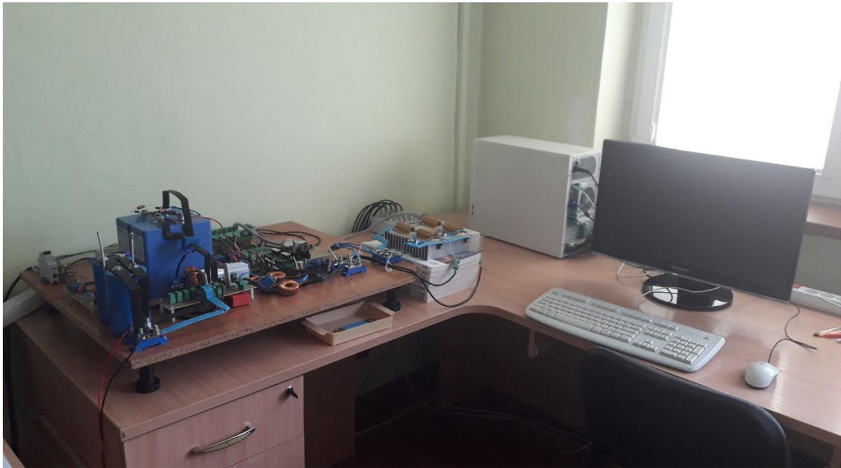
Figure 1. Laboratory stand of buck DC-DC power converter with low damped input LC filter.
