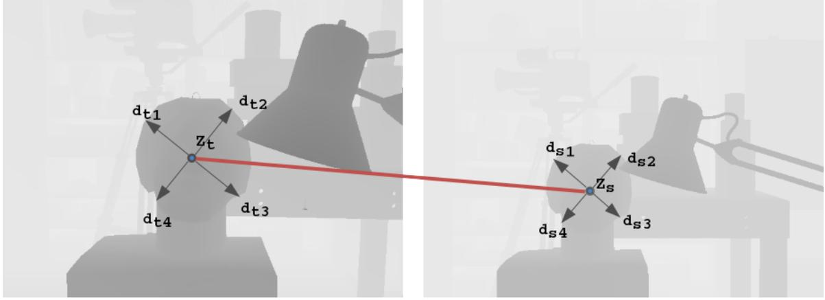
Figure 1: Comparison of distances  $d_t$ ,  $d_s$  to the nearest edges for all rays determined for keypoints in the template image and scene images correspondingly. Disparity maps come from dataset [5]
