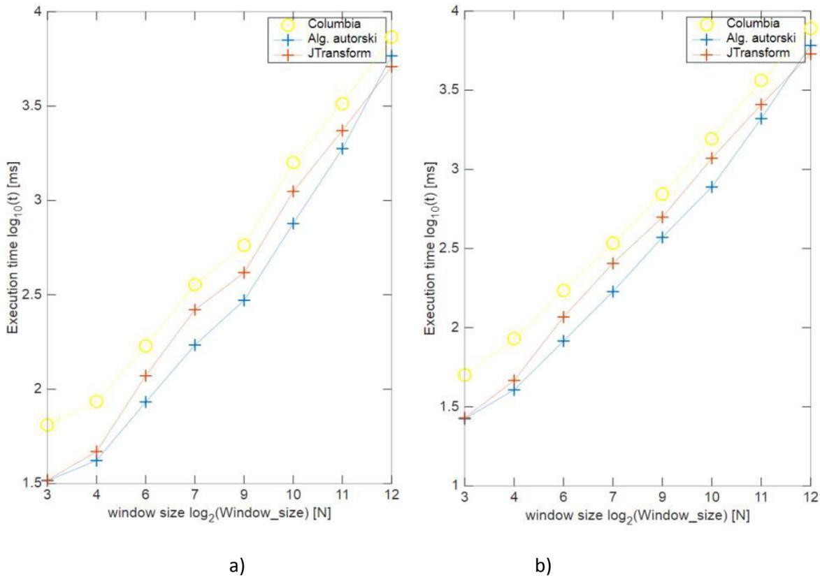
Figure 2. Analysis of execution times of frequency transform algorithms taking into account the warm up effect (a- average execution time for all iterations, b - average execution time of algorithms without taking into account the first five iterations)
