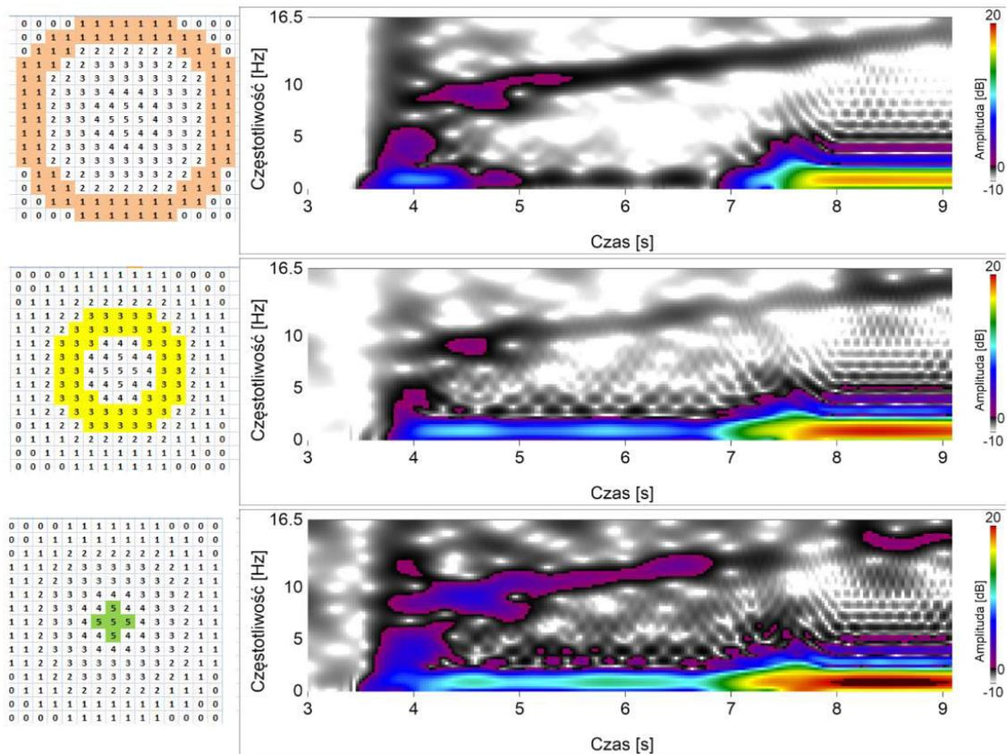
Figure 3. Spectrograms for tomographic data - rings R1, R3, R5 (h = 150 cm; smooth wall; filling: funnel)
